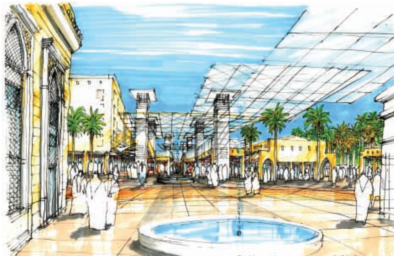
The Main Souk incorporates solar panels for shading, fountains for evaporative cooling and solar chimneys to create breeze without using energy
