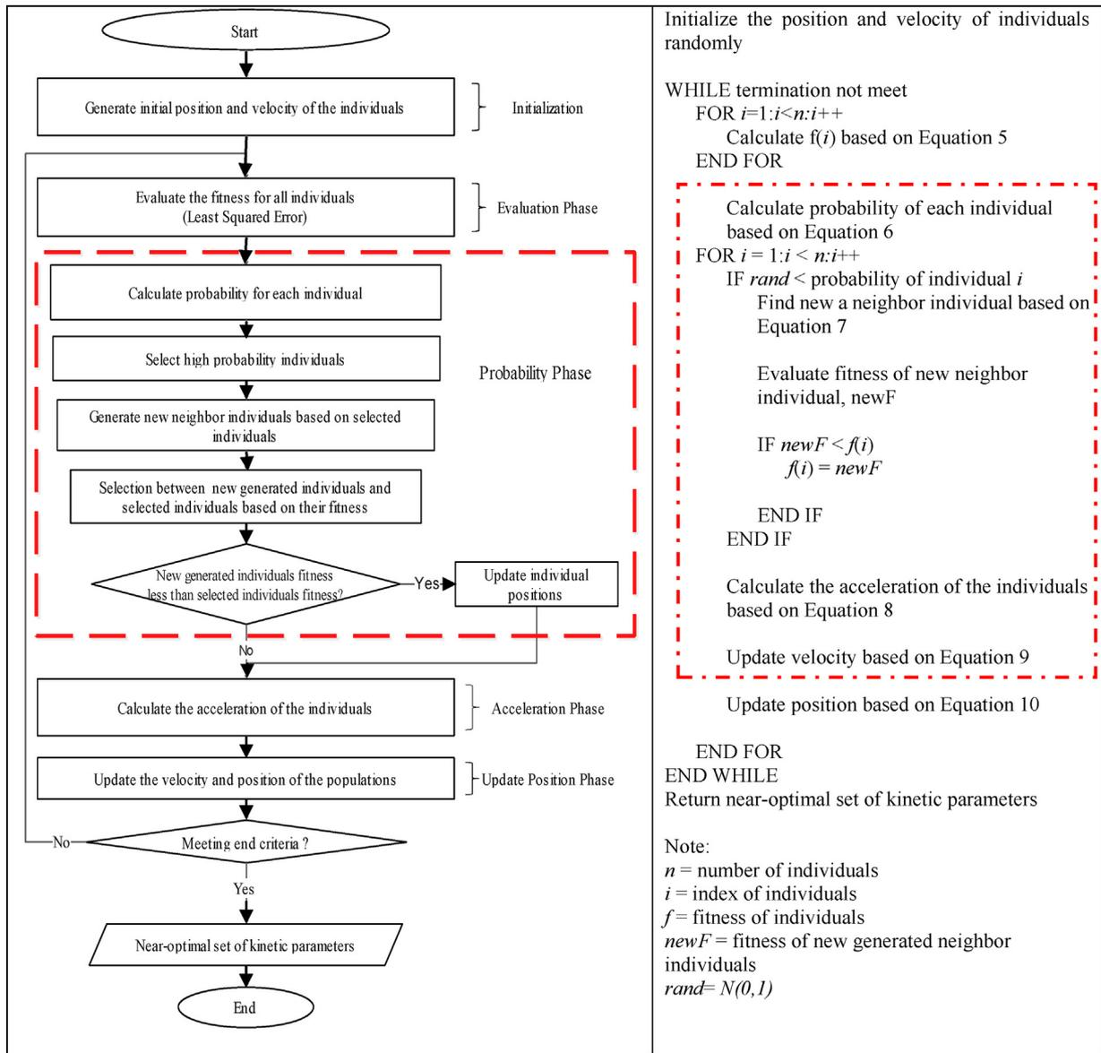
Fig. 1. The flowchart and pseudocode of IPSOGSA (Note: Dotted line describes the improved part).
