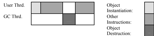
Figure 3. Current memory management model: GC thread works with non-deterministic behavior.
